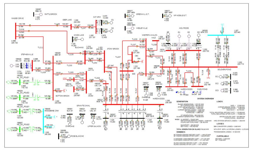
Figure 2 - IIS (2030 High Load Conditions – ML Firm Exports (250 MW))
