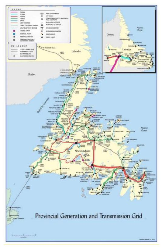
Figure 1 : Newfoundland and Labrador Interconnected System
