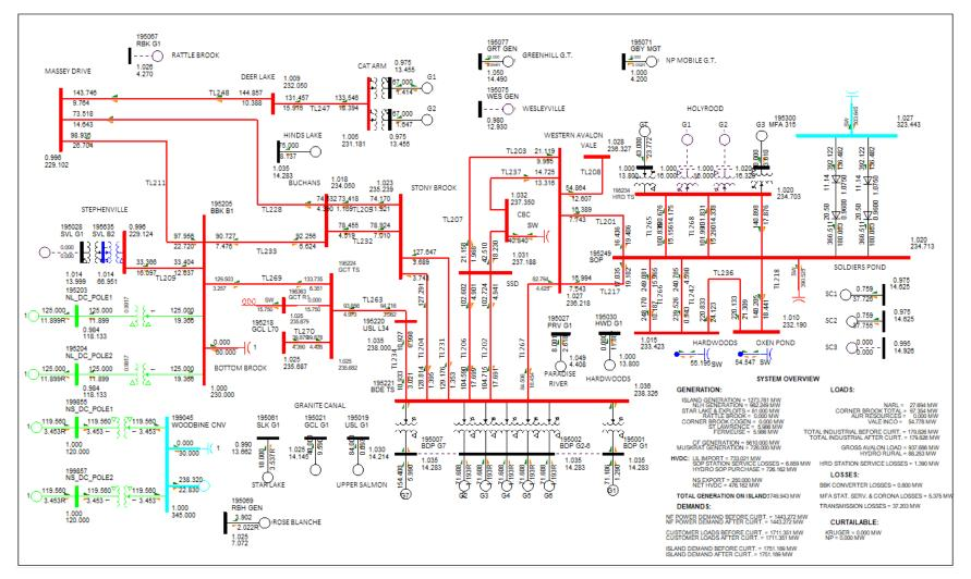
Figure 3 - IIS (2030 High Load Conditions – ML Firm Exports (250 MW))
